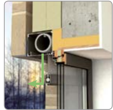
Installation method 7 (100 EVO )
